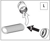
• Fit the end of the hose 12 to the wall flange 11 as shown in fig. M.
